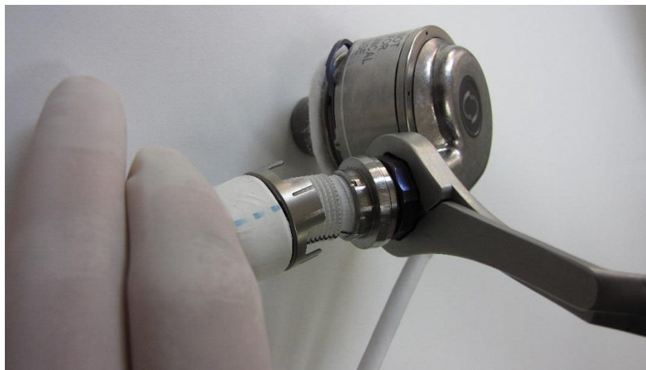
Figure 16 – Aligned jaws fully clamped on the socket profile.
