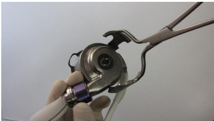
Figure 5 – A2 Open the clamps jaws and firmly grab the object
