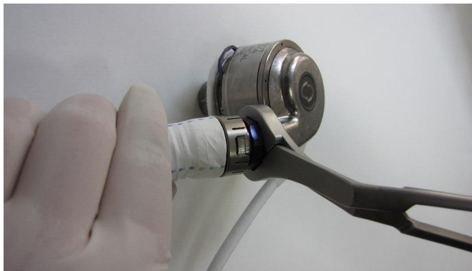
Figure 17 - Connecting the protective tube of the outflow graft onto the outflow graft socket.
