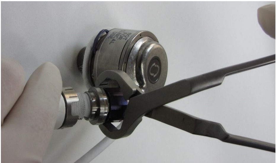
Figure 15 – A2 Opening the jaws and clamping the socket.
