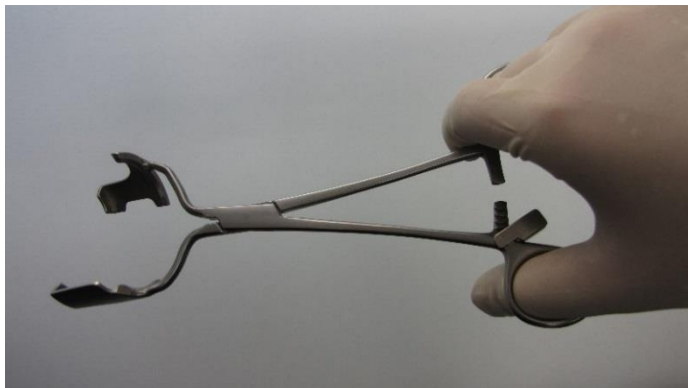
Figure 4 – A1 Unlock the locking cover on the clamps and verify the motion range.
